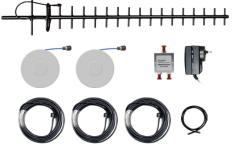
This kit features the Blackhawk YAGI 14dBi antenna which is affixed on the rooftop collecting the mobile signal from outside and transferring it to Cel-Fi GO. The 4-6dBi indoor pulse DAS antennas, spaced out at 20m apart, boost the signal internally, covering large areas.
